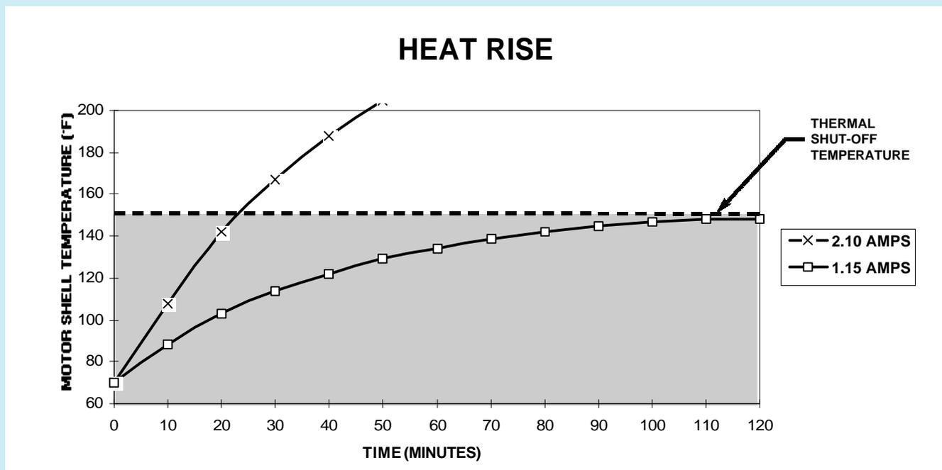
The shaded area in both the Performance Data and Heat Rise charts, contains pumps with current levels that are capable of running without periodic cool down. Pumps in this category will generally transfer more water over sustained periods than those in the unshaded areas, which are required to shut down while the motor cools. Some applications require maximum flows at high pressures for relatively short periods, however, so an explanation of thermal protection follows:
